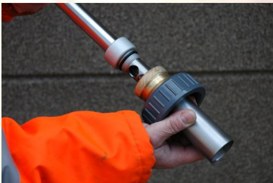
Mount the flow direction meter onto the proper adapter.
