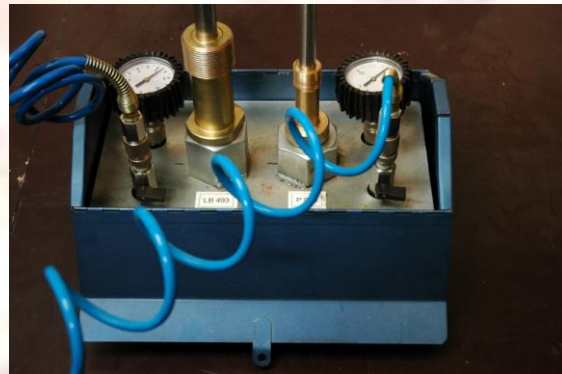
Testing of hot tap tools
