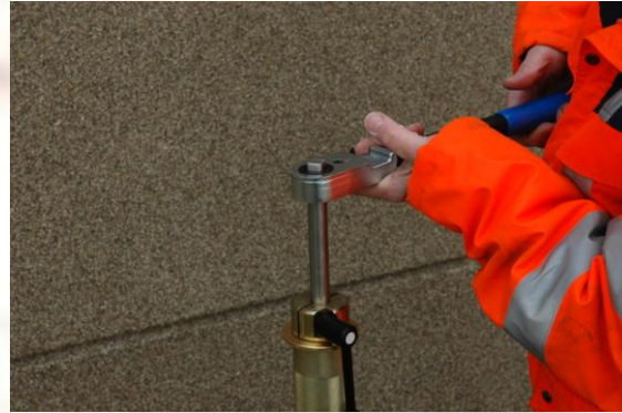
Retrieve the drilling spindle
