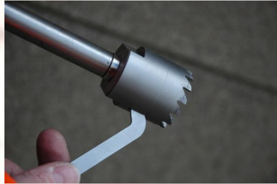
Removal of cutted coupon
