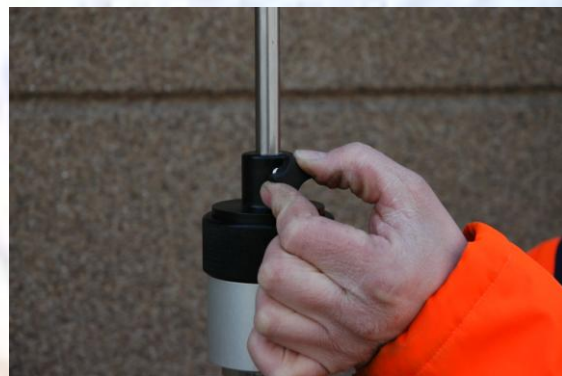
Untighten the locking screw of the gauge rod.
