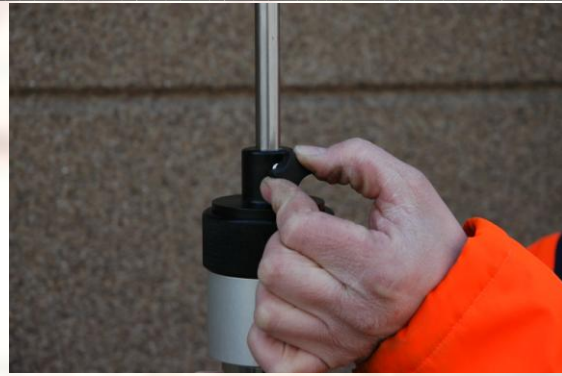
Check whether the gauge rod is in complete upwards position and is secured by means of the screw. Otherwise the gauge rod may fall down..
