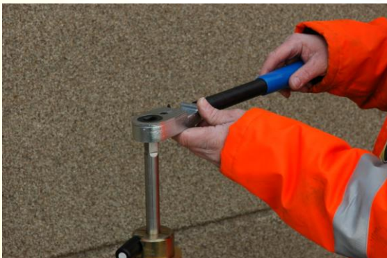
Install the ratchet onto the the drilling spindle.
