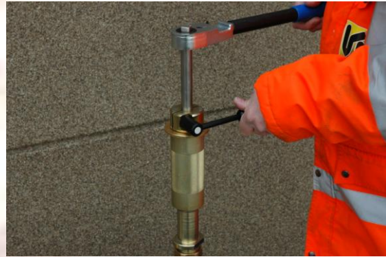
After you retrieved the spindle completely, lock the lever again.
